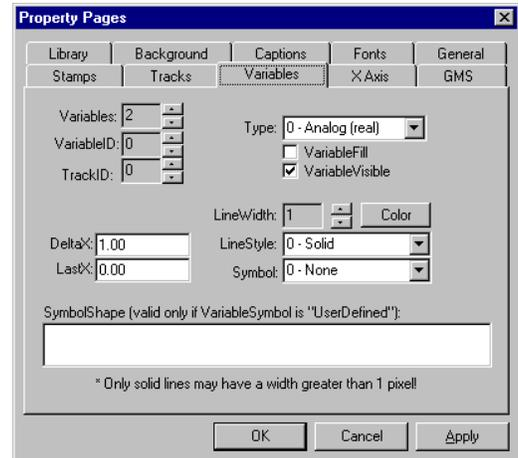
Figure 12 - Trending ActiveX Control Property Configuration Form with Tabbed Dialog Box
