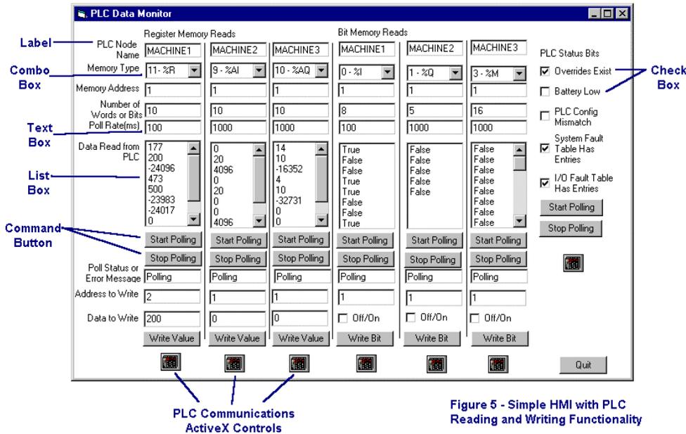
Figure 5 - Simple HMI with PLC Reading and Writing Functionality
