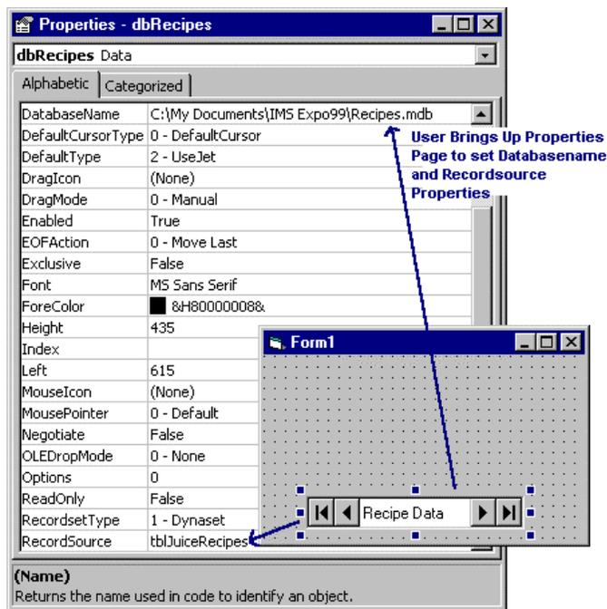
Figure 3 - Database Connectivity Using Data Control
