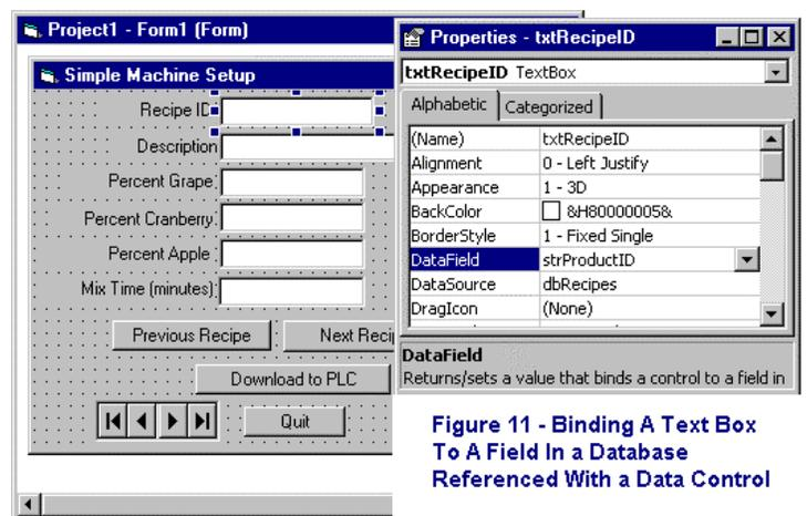
Figure 11 - Binding A Text Box To A Field In a Database Referenced With a Data Control
