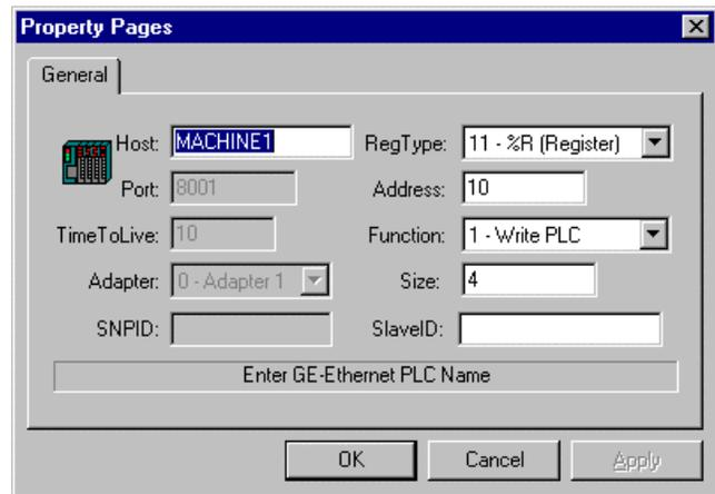
Figure 10 - PLC ActiveX Control Property Configuration Dialog Box
