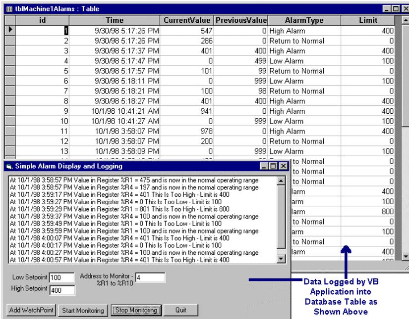
Figure 14 - Alarming Application Showing VB Application Screen and Data As Logged in the Database
