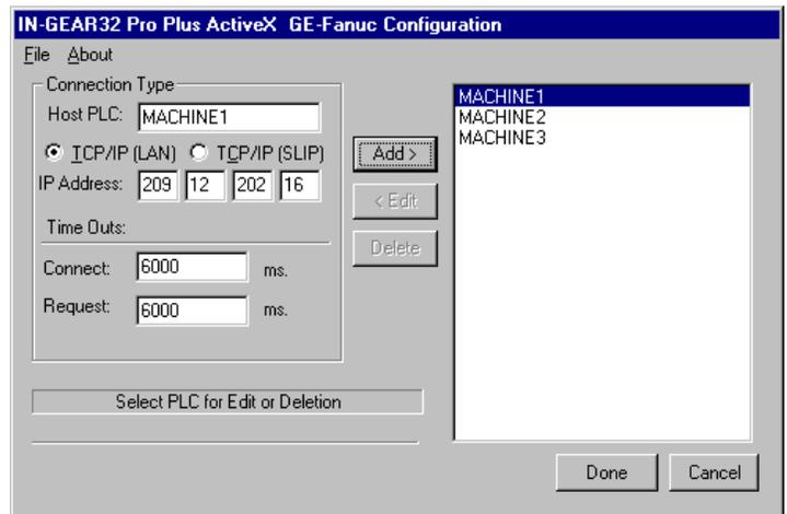
Figure 6 - Utility for Configuring Physical PLC Connections
