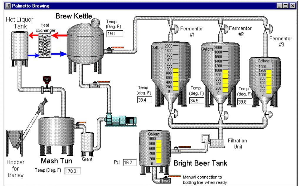
Figure 8 - An HMI Screen Developed for A Micro-brewery Application
